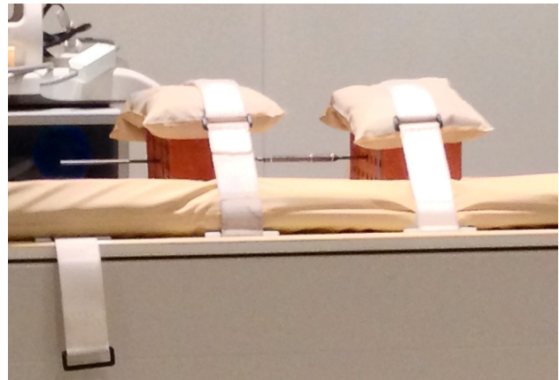
Fig. 1 MCGR held in a ceramic jig secured within the gantry of the 1.5 T Phillips magnetic resonance imaging scanner
