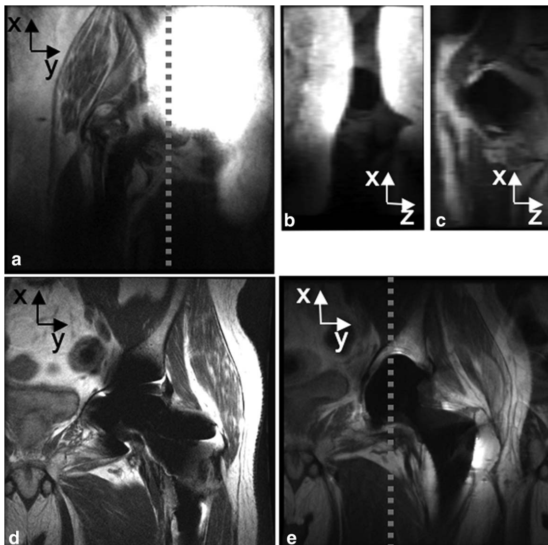
FIG. 6. Clinical utility of the VS-3D-MSI method on total hip replacements. a: MAVRIC image of a total hip replacement where through-plane aliasing overwhelms the signal near the implant. b: Reformat (coordinate axes indicate logical encoding directions) of the MAVRIC image displayed in (a), indicated through dotted line. c: Reformat of a VS-3D-MSI image on another total hip replacement patient where the aliased signal seen in (b) has now been removed. d: In-plane 2D-FSE image of the implant displayed in (c). e: In-plane VS-3D-MSI image of the case displayed in (d), with dotted line indicating the position of the reformatted image in (c). In-plane ( k_y ) aliasing remains in the VS-3D-MSI image (e), but is suppressed in the clinical 2D-FSE images (d) via the application of extra phase encodes embedded in the signal-averaging process (i.e., k_y oversampling).
