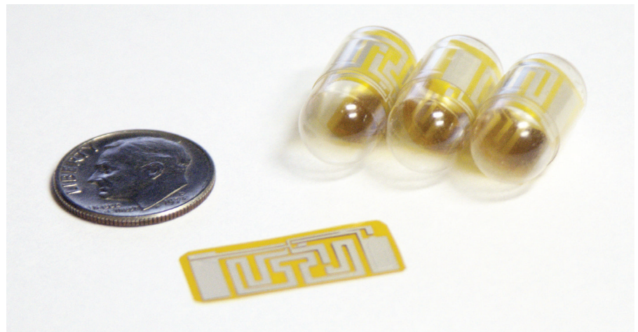
E-detecting. This wireless tracking device, which is embedded into a standard gelatin capsule, communicates with an external hub. Source: Glen Flores, eTect Inc.
